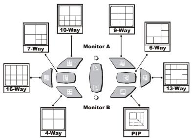
The multiscreen display is limited to the number of camera inputs on the unit.
